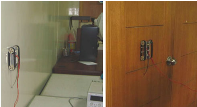
Fig. 11.5 A gecko-inspired robot is shown climbing vertical walls of different materials. Vertical climbing is enabled with the robot's polyurethane micro-hair array on its wheels (Wu et al. 2013). (Images provided courtesy of Springer)
