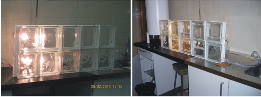
Fig. 7.10 Glass block photo-bioreactor. Lab tests
